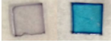
Figure 11. Sensors made with PAB. (Left) Exposed to kerosene only. (Right) Exposed to 10,000 ppm (v/v) phenol.
